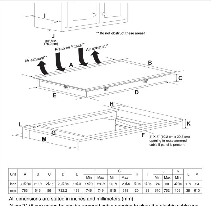
Allow 2'' (5 cm) space below the armored cable opening to clear the electric cable and allow space for installation of the junction box on the wall at the back of the cooktop.
